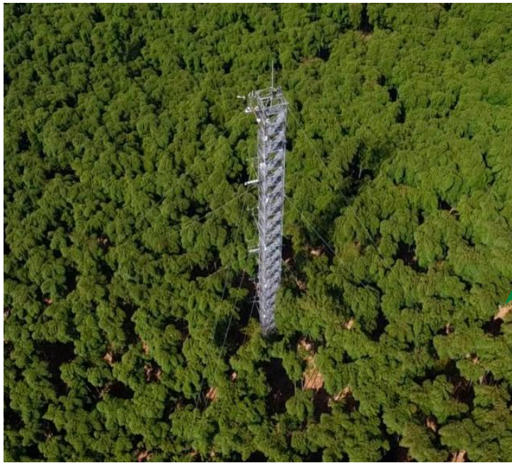
Ecosystem carbon flux of Moso bamboo monitored by the eddy covariance tower in Anji, Zhejiang
